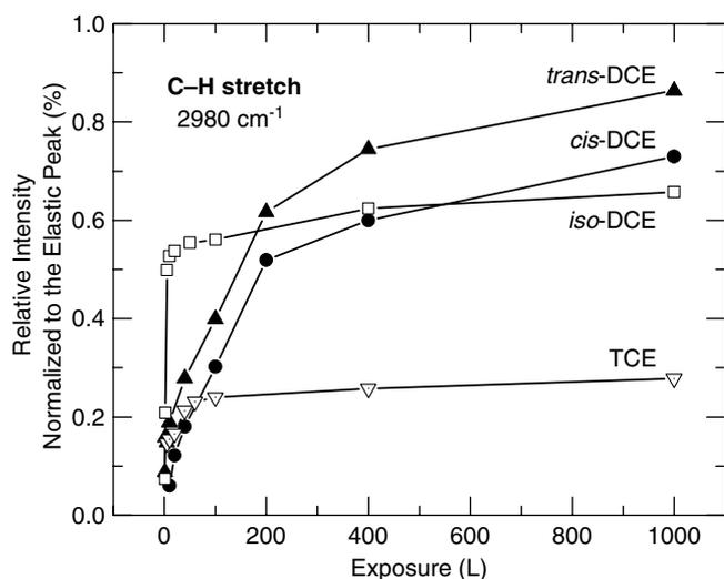
Fig. 3. Exposure dependence of the relative intensities of the C–H stretch normalized to the respective elastic peaks for *iso*-, *cis*- and *trans*-dichloroethylene (DCE) and trichloroethylene (TCE) on Si(111)7 × 7 at room temperature.
