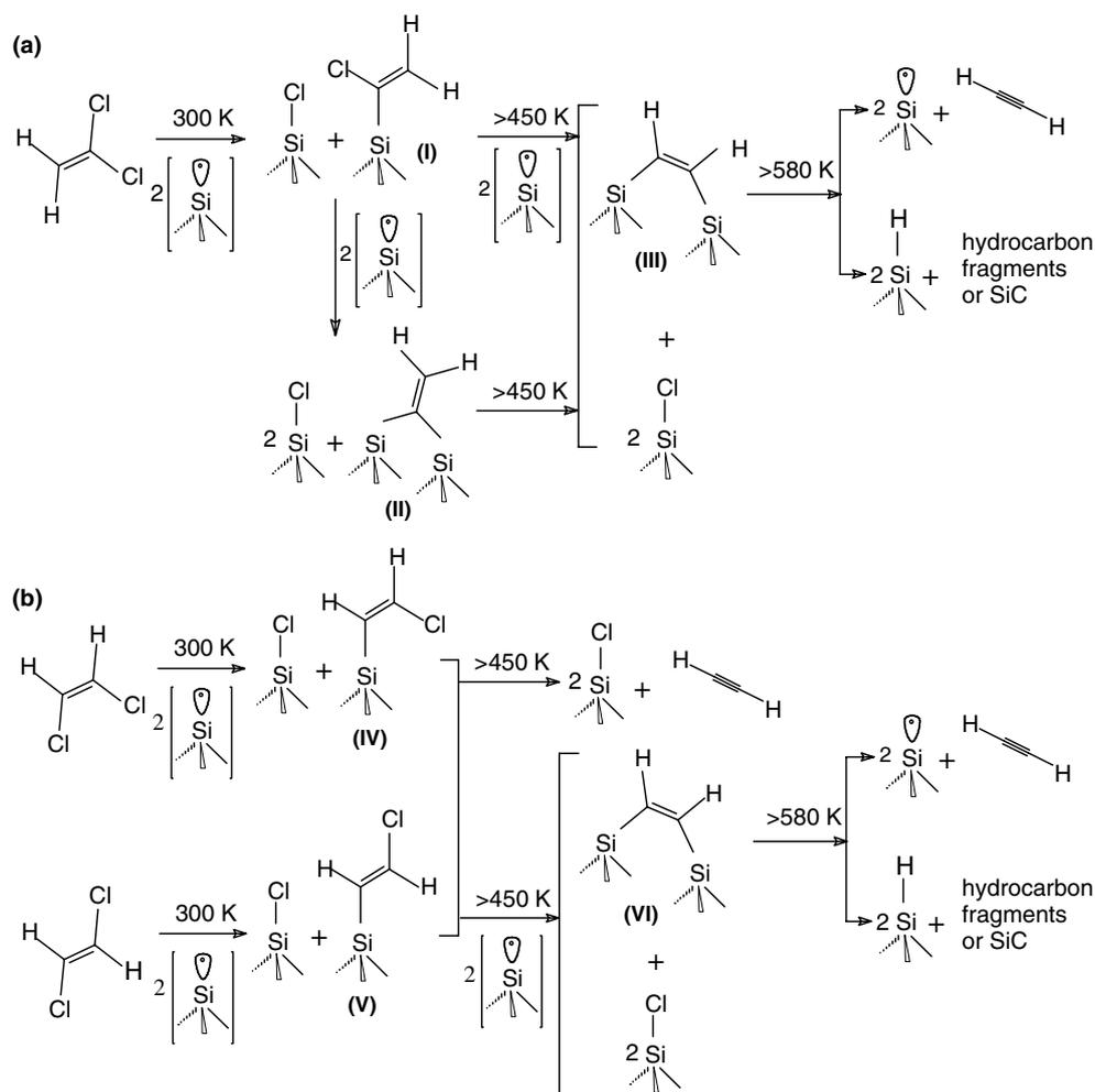
Fig. 2. Schematic diagrams of plausible adsorption structures and thermal evolution products for saturation exposures of (a) *iso*-dichloroethylene, and (b) *cis*- and *trans*-dichloroethylene to Si(111)7 $\times$ 7 at room temperature.
