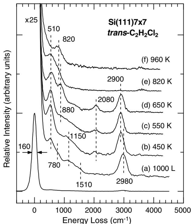
Fig. 7. Vibrational electron energy loss spectra for 1000 L of *trans*-dichloroethylene exposed to (a) Si(111) $7 \times 7$  at room temperature, and upon annealing to (b) 450 K, (c) 550 K, (d) 650 K, (e) 820 K, and (f) 960 K.
