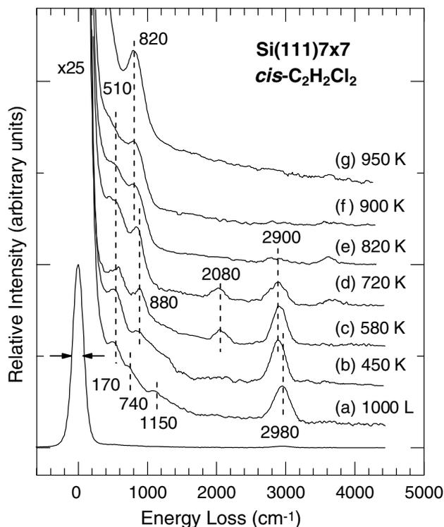
Fig. 6. Vibrational electron energy loss spectra for 1000 L of *cis*-dichloroethylene exposed to (a) Si(111) $7 \times 7$  at room temperature, and upon annealing to (b) 450 K, (c) 580 K, (d) 720 K, (e) 820 K, (f) 900 K and (g) 950 K.
