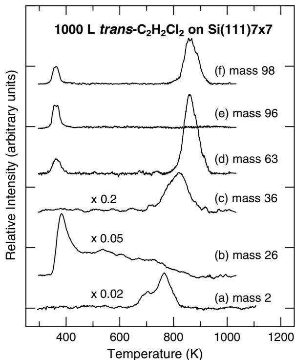
Fig. 5. Thermal desorption profiles of (a) mass 2 ( $\text{H}_2^+$ ), (b) mass 26 ( $\text{C}_2\text{H}_2^+$ ), (c) mass 36 ( $\text{HCl}^+$ ), (d) mass 63 ( $\text{C}_2\text{H}_2^{37}\text{Cl}^+$  or  $\text{Si}^{35}\text{Cl}^+$ ), (e) mass 96 ( $\text{C}_2\text{H}_2^{35}\text{Cl}_2^+$ ), and (f) mass 98 ( $\text{C}_2\text{H}_2^{35}\text{Cl}^{37}\text{Cl}^+$  or  $\text{Si}^{35}\text{Cl}_2^+$ ) for 1000 L of *trans*-dichloroethylene exposed to  $\text{Si}(100)7 \times 7$  at room temperature.
