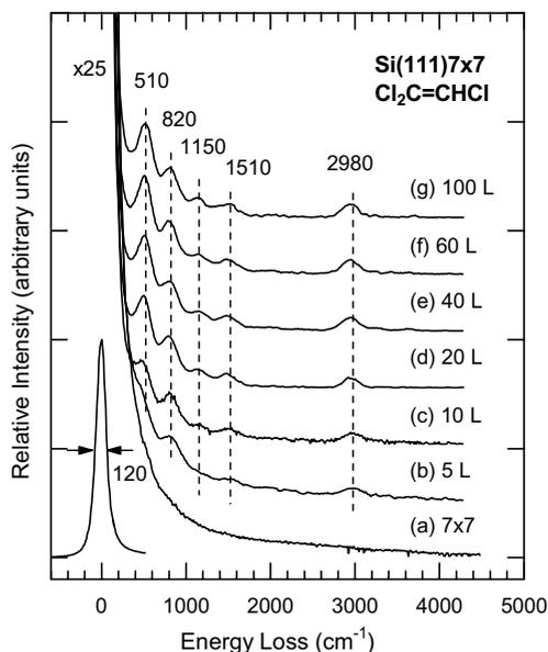
Fig. 2. Vibrational electron energy loss spectra for trichloroethylene exposed to (a) Si(111)7 × 7 at room temperature as a function of exposure: (b) 5 L, (c) 10 L, (d) 20 L, (e) 40 L, (f) 60 L, and (g) 100 L.
