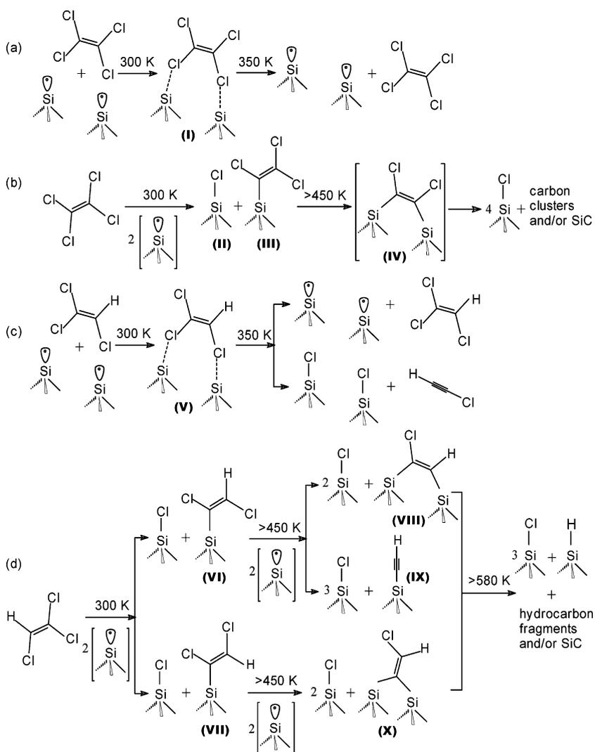
Fig. 7. Schematic diagrams of plausible adsorption structures and thermal evolution products for (a,b) perchloroethylene and (c,d) trichloroethylene exposed to Si(111)7 $\times$ 7 at room temperature.
