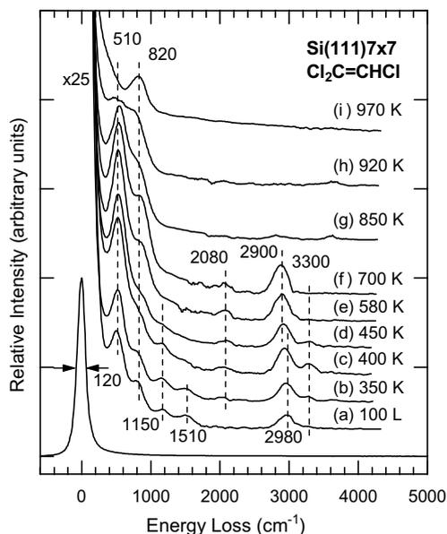
Fig. 6. Vibrational electron energy loss spectra for 100 L of trichloroethylene exposed to (a) Si(111)7 × 7 at room temperature, and upon annealing to (b) 350 K, (c) 400 K, (d) 450 K, (e) 580 K, (f) 700 K, (g) 850 K, (h) 920 K, and (i) 970 K.
