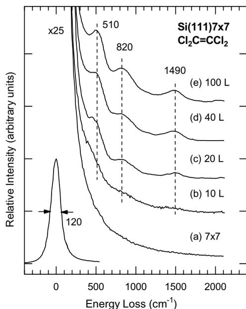
Fig. 1. Vibrational electron energy loss spectra for perchloroethylene exposed to (a) Si(111)7×7 at room temperature as a function of exposure: (b) 10 L, (c) 20 L, (d) 40 L, and (e) 100 L.
