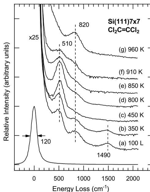
Fig. 5. Vibrational electron energy loss spectra for 100 L of perchloroethylene exposed to (a) Si(111) $7 \times 7$  at room temperature, and upon annealing to (b) 350 K, (c) 450 K, (d) 800 K, (e) 850 K, (f) 910 K, and (g) 960 K.
