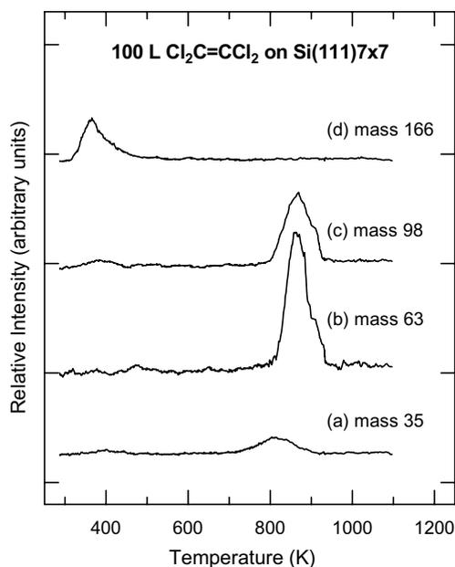
Fig. 3. Thermal desorption profiles of (a) mass 35 ( $\text{Cl}^+$ ), (b) mass 63 ( $\text{SiCl}^+$ ), (c) mass 98 ( $\text{SiCl}_2^+$ ), and (d) mass 166 ( $\text{C}_2\text{Cl}_3^+$ ) for 100 L of perchloroethylene exposed to  $\text{Si}(100)7\times 7$  at room temperature.
