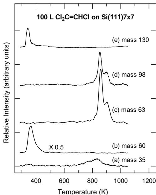
Fig. 4. Thermal desorption profiles of (a) mass 35 ( $\text{Cl}^+$ ), (b) mass 60 ( $\text{C}_2\text{HCl}^+$ ), (c) mass 63 ( $\text{SiCl}^+$ ), (d) mass 98 ( $\text{SiCl}_2^+$ ), and (e) mass 130 ( $\text{C}_2\text{HCl}_3^+$ ) for 100 L of trichloroethylene exposed to  $\text{Si}(111)7 \times 7$  at room temperature.
