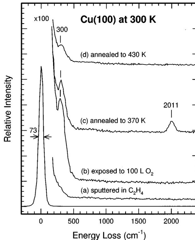
Fig. 7. Vibrational electron energy loss spectra for (a) Cu(100) sputtered in  $1 \times 10^{-6}$  Torr of ethylene at 50 eV and 10 nA/mm<sup>2</sup> for 10 minutes at 300 K, and (b) sample (a) exposed with 100 L of O<sub>2</sub>, followed by annealing to (c) 370 and (d) 430 K.
