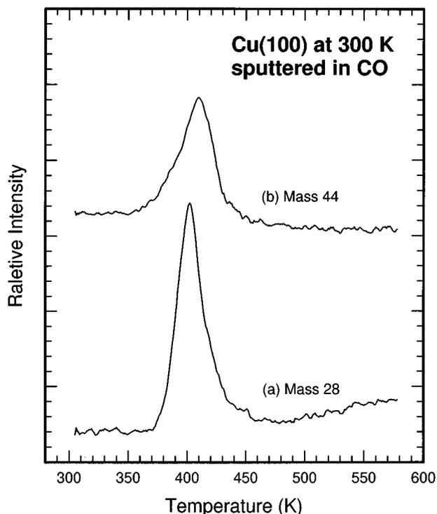
Fig. 5. TPD profiles of (a) mass 28 and (b) mass 44 for Cu(100) sputtered in  $1 \times 10^{-6}$  Torr of CO at 200 eV and  $10 \text{ nA/mm}^2$  for 10 minutes at 300 K. The linear heating rate was 1 K/s.
