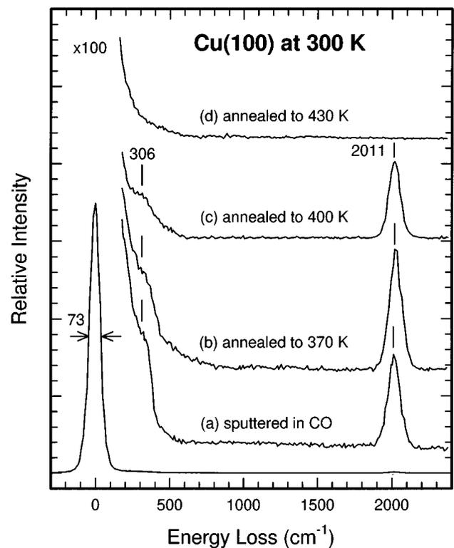
Fig. 4. Vibrational electron energy loss spectra for (a) Cu(100) sputtered in  $1\times 10^{-6}$  Torr of CO at 200 eV and  $10\text{ nA}/\text{mm}^2$  for 10 minutes at 300 K, followed by annealing to (b) 370, (c) 400, and (d) 430 K.
