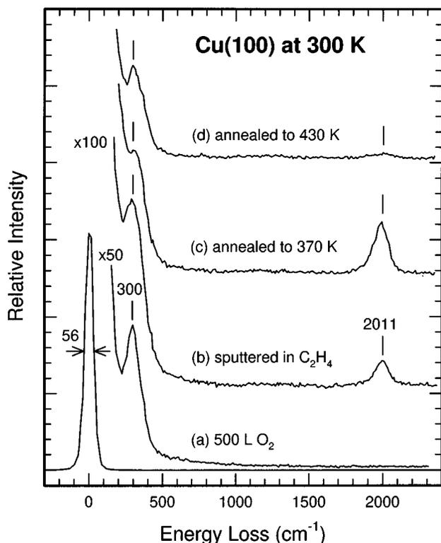
Fig. 6. Vibrational electron energy loss spectra for (a) Cu(100) exposed with 500 L of O<sub>2</sub> at 300 K, and (b) sample (a) sputtered in  $1 \times 10^{-6}$  Torr of ethylene at 50 eV and 10 nA/mm<sup>2</sup> for 10 minutes, followed by annealing to (c) 370 and (d) 430 K.
