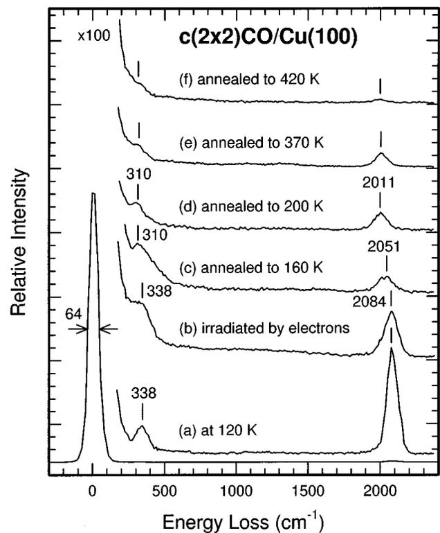
Fig. 3. Vibrational electron energy loss spectra for (a) 100 L of CO adsorbed on Cu(100) at 120 K, and (b) sample (a) irradiated with electrons at 100 eV and  $2.7\text{ }\mu\text{A}/\text{mm}^2$  for 10 minutes at 120 K, followed by annealing to (c) 160, (d) 200, (e) 370, and (f) 420 K.
