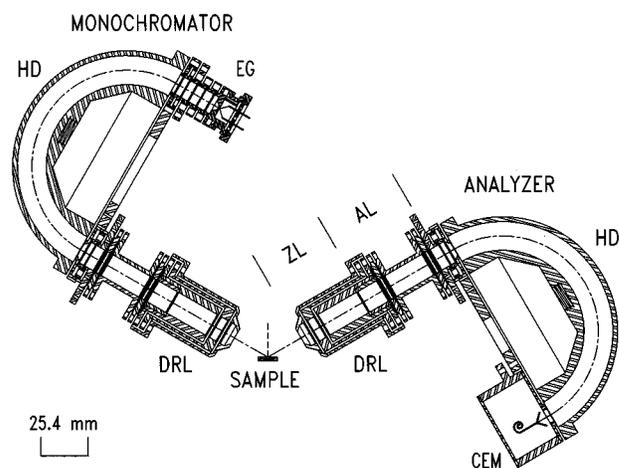
Fig. 1. Schematic diagram of the electron energy loss spectrometer at the University of Waterloo. EG: electron gun; HD: hemispherical deflector; DRL: double retardation lens; ZL: zoom lens; AL: afocal lens, CEM: channel electron multiplier.
