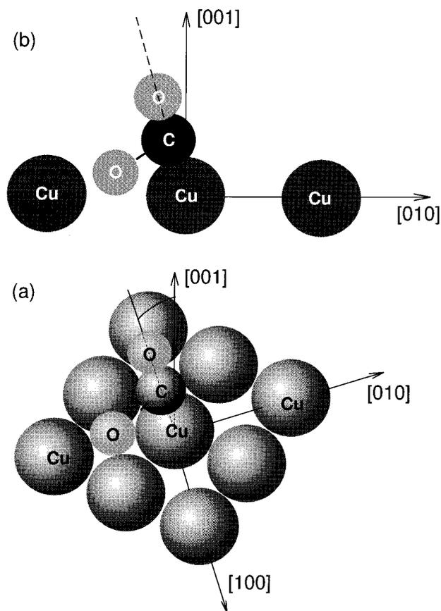
FIG. 8. Perspective (a) and side view (b) diagrams of a proposed bonding structure for CO coadsorbed with O on Cu(100).
