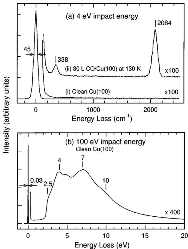
Fig. 2. Typical electron energy loss spectra for (a) a clean Cu(100) surface with (ii) and without (i) a 30 L exposure of CO at 130 K collected at 4 eV impact energy, and for (b) a clean Cu(100) surface recorded at 100 eV impact energy over an extended energy loss range illustrating the onset of the electronic band structure.
