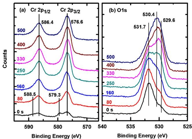
FIG. 3. (Color online) XPS spectra of (a) Cr  $2p$  and (b) O  $1s$  regions of a  $\text{CrO}_2$  film as grown on  $\text{MgO}(100)$  at  $480^\circ\text{C}$  with 400 mTorr  $\text{O}_2$  pressure and upon sputtering for 80, 160, 250, 330, 400, and 500 s.
