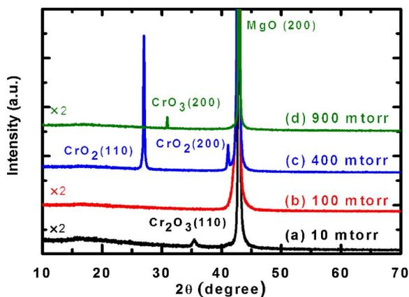
FIG. 1. (Color online)  $2\theta$ - $\omega$  XRD spectra for the  $\text{CrO}_x$  films grown on  $\text{MgO}(100)$  substrates at  $\text{O}_2$  pressure of (a) 10 mTorr, (b) 100 mTorr, (c) 400 mTorr, and (d) 900 mTorr. The intense feature at  $2\theta=42.9^\circ$  corresponds to the  $\text{MgO}(200)$  substrate peak.
