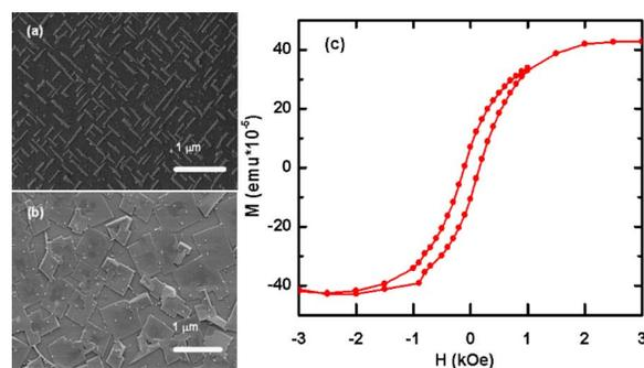
FIG. 2. (Color online) SEM images of a  $\text{CrO}_2$  film grown at 480 °C with 400 mTorr  $\text{O}_2$  pressure, depicting both (a) nanoneedles near the edges and corners of the sample, and (b) plates near the film center. (c) shows the magnetization ( $M$ ) vs field ( $H$ ) curve at 5 K, with  $H$  parallel to the film surface. The paramagnetic contribution has been subtracted from the curve.
